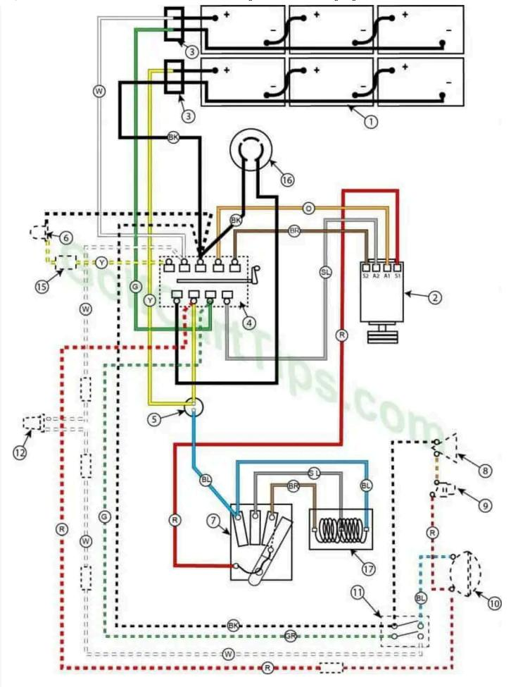
The 1957 36-volt Golfster and Industrial have one selector switch, now with a "Charge" setting. They have a three belt drive and a twist-lock external charging plug. It is now equipped with two battery racks.
