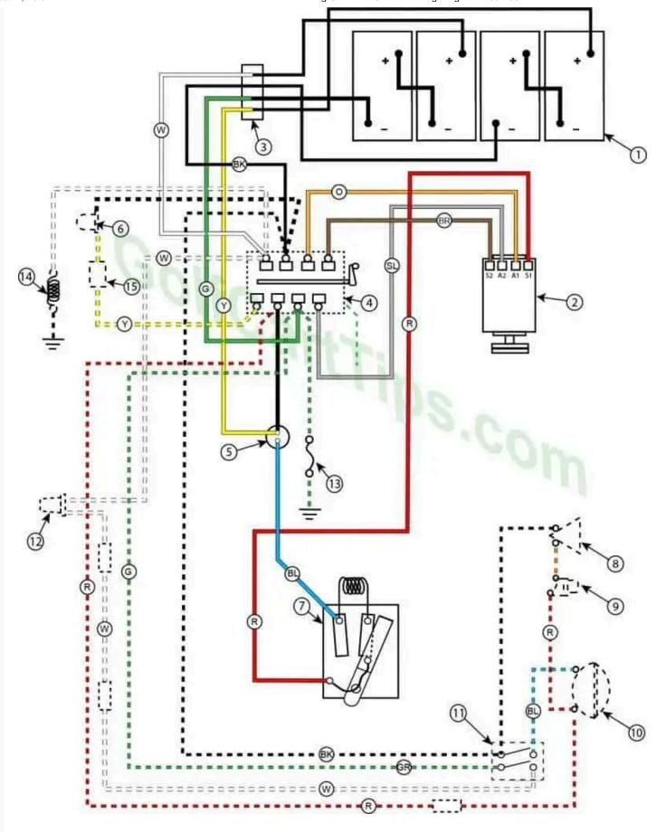
Dashed lines indicate the accessory wiring.
