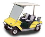
The Town and Fairway model was also introduced in 1968 and sported a 4-seater with the 3rd and 4th seat facing backward. This version came in either 36 volt electric or with a 10hp Kohler K241 engine. From 1974 to 1975, the Combo 1 version of the Town and Fairway was produced which featured the ability to fold down the back passenger seat for golf bags. There were only 200-300 of these built.
